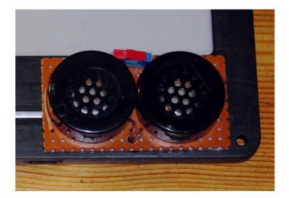
At the top of the board a small slide switch which was mounted on the stripboard to cut the speakers can be seen. It is not intended to be used in flight but I wanted to be able to cut the audio when using the unit on the ground for retrieve or rescue purposes.
