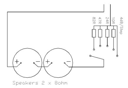
The switch I use is a 2 pole 6 way PCB mounting switch AB 417 Conrad part No. 705683-62. The resistor values in the diagram give a change of volume of about 4dB per step with a 16 ohm speaker. The bottom position is completely off.
